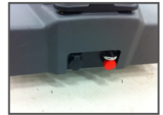
Foot activated emergency stop button and magnetic charger port.
